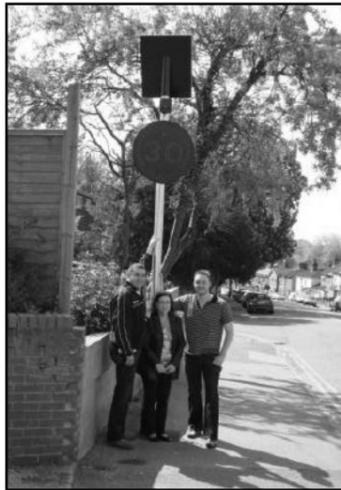
A new Vehicle Activated sign (VAS) has been installed near Rectory Close on Mile End Road. The sign has already been proven to help reduce traffic speeds.
